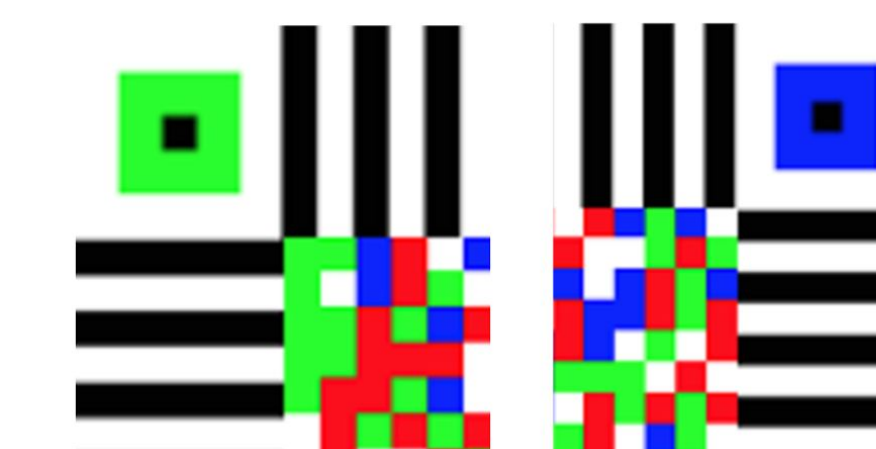
Fig. 2: Close-up of our top left and right corners and timing strips
