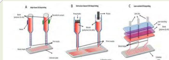
Figure 1: 3D bioprinting technologies. (A) Inkjet-based 3D bioprinting, (B) Extrusion-based 3D bioprinting, (C) Laser-based 3D bioprinting [1].
