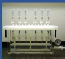
Solid Phase Extraction System, containing cartridges
