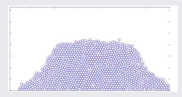
Collision Generator: N= 1024 particles, Solver = MinMap Netwon, Tolerance = 1E-9
